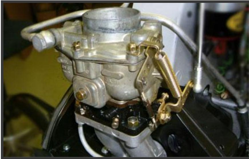
Remove the accelerator pump links (#8). This is simple enough on the right hand carb, but the left is more difficult. Similarly, access to the main and idle jets (parts 67 and 68) is not easy on either carb, as-installed. You can R&R the carb(s) if you find it easier than working in place, but they will require R&Ring in the plural.
